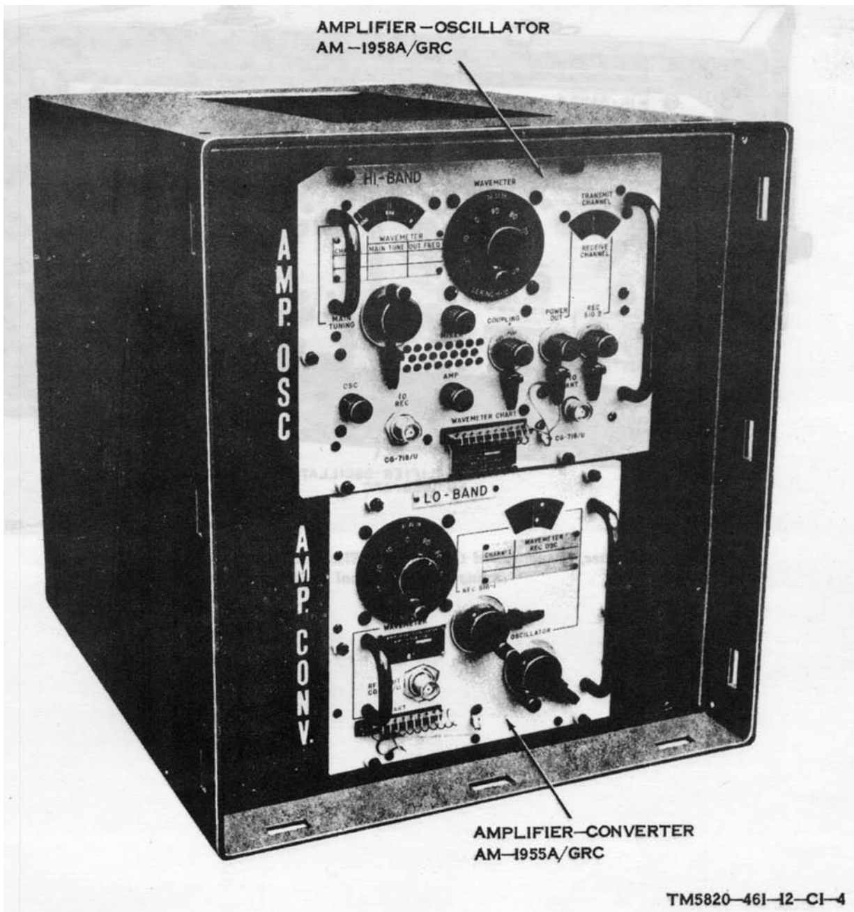
Figure 1-13.1. Case, Standardized Components, Electrical CY-2582/GRC with alternate tuning heads; later design
